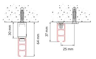
Ceiling mounting with mini suspension hanger
